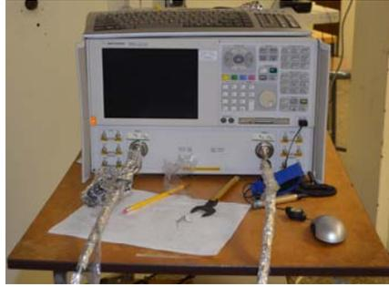
Figure 6: Agilent E8363B Vector Network Analyzer
