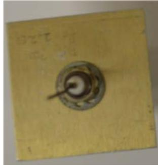
(b) Monopole Antenna Working at 2.25 GHz
