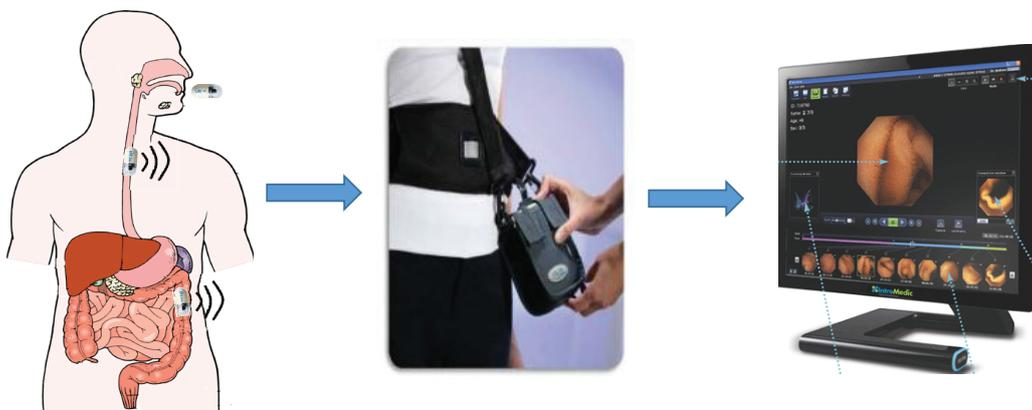
Figure 2.3: The procedure of wireless capsule endoscopy: (a) swallow WCE, going through GI tract and transmitting images; (b) outside receivers receives images and transfers those pictures to medical workstation; (c) physicians take over the medical reviews and make decisions
