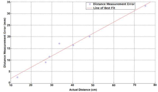
Figure 6: Distance Measurement Error from TOA for each sensor position
