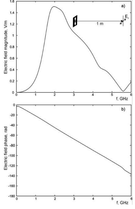
Radiated electric field (the y-component) as a function of frequency at a distance of 1 m from the transmitting antenna: a) – magnitude; b) – phase.
