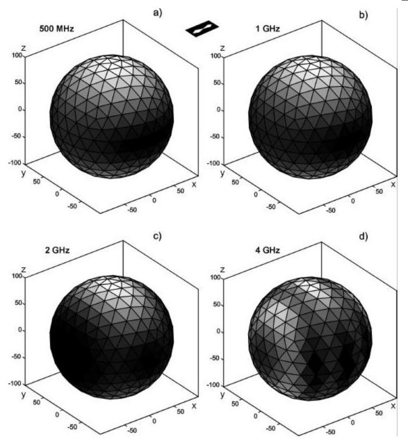
Radiation intensity distribution over the sphere surface with the radius of 100 m at four different frequencies.
