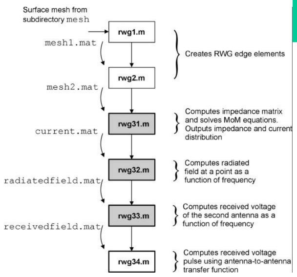
Flow chart for the time-domain analysis. Scripts containing frequency loop are grayed.
