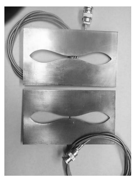
Slot antenna of Time Domain, Inc., linearly polarized, without reflector
