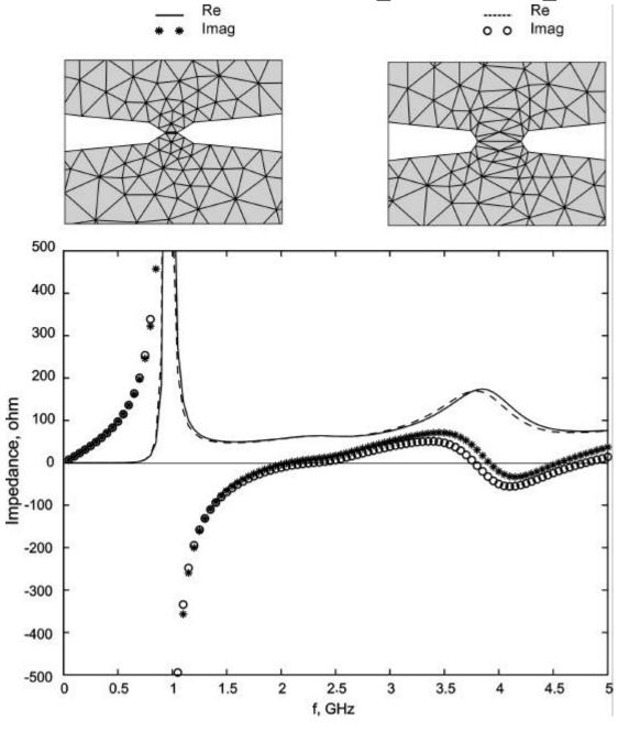
Input impedance as a function of frequency for two different feed models. Solid and dashed lines show the input resistance. The input reactance is shown by stars and circles, respectively.
