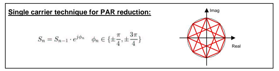
OFDM with DFT spreading and  $\pi$ /4-QPSK subcarrier modulation:
