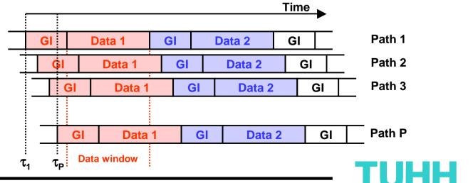
Broadband OFDM-FDMA System for the Uplink of a Wireless LAN
