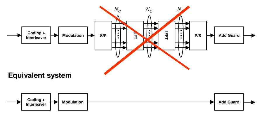
An OFDM system with DFT spreading is equivalent to a single-carrier system with guard interval
