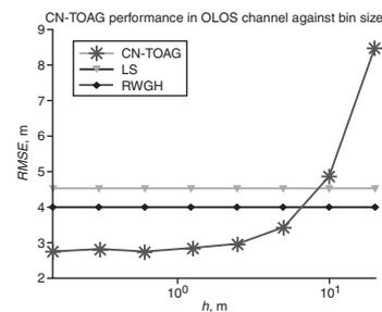
Fig. 2 Comparison of CN-TOAG performance against LS and RWGH algorithms
