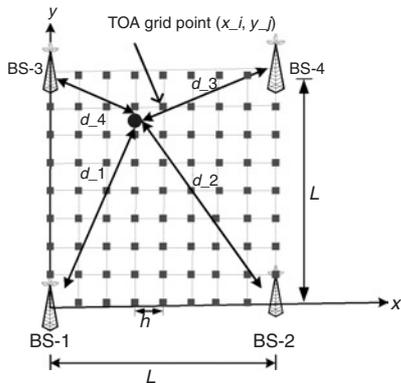
Fig. 1 Geolocation system showing TOA grid for CN-TOAG algorithm
