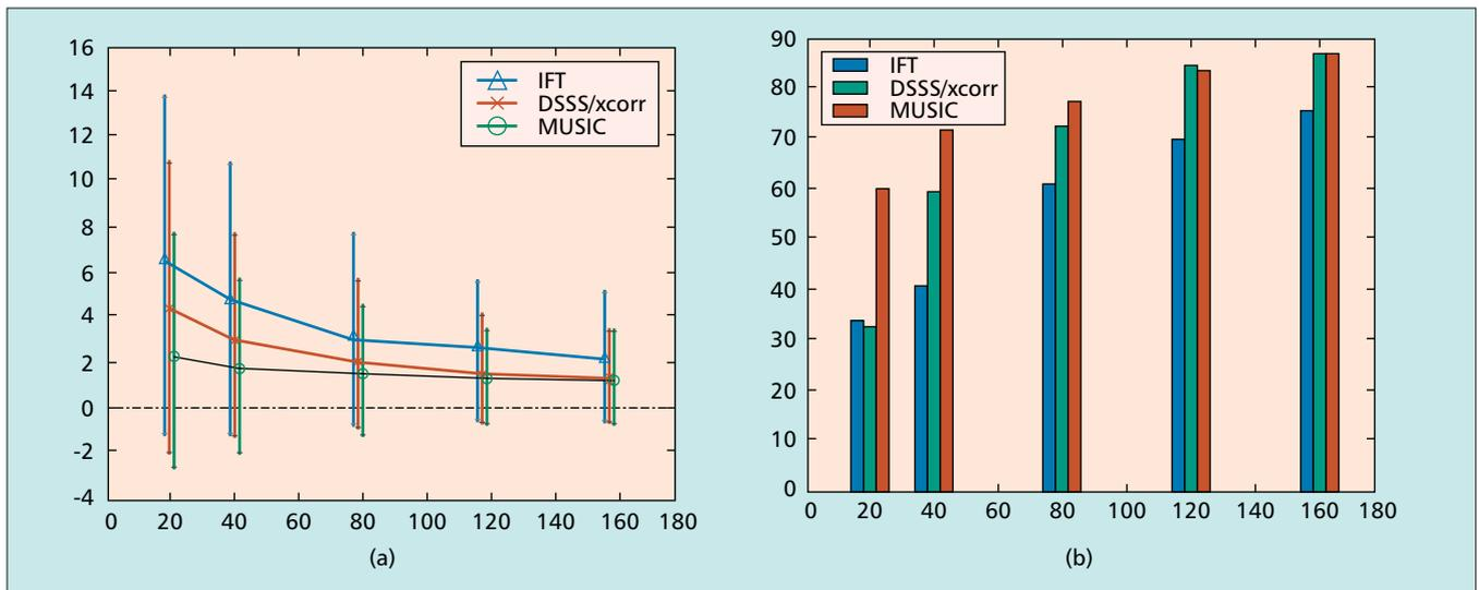
■ **Figure 4.** Simulation results: a) mean of ranging errors in meter vs. bandwidth in MHz using three different TOA estimation techniques; the vertical line corresponds to one standard deviation; b) percentage of measurement locations where absolute ranging errors are smaller than 3 m vs. bandwidth in MHz.
