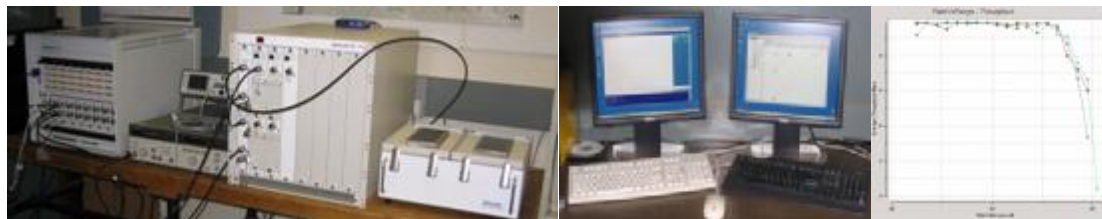
Figure 3: RF isolated multipath testbed at CWINS using Azimuth RF chamber and PROPSIM real time channel simulator.
